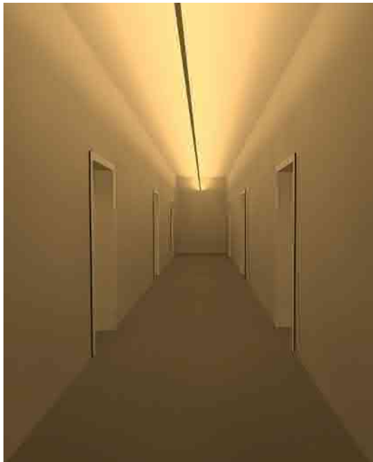
LED Strip :2000lm/meter.17.9w/m.View angle:120degree. Ra>80.3000K
